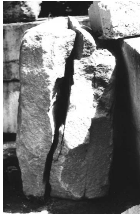
Fig. Very hard rubble stone crushed by electro-hydraulic explosion
