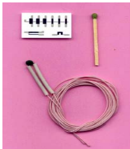
Fig. 1. View of planar-type thick-film thermistors of different topology and disk-type bulk analogue, for comparison
