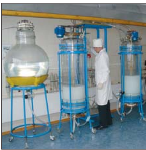
Pilot line for nanopowder manufacturing. Chemical zone.
