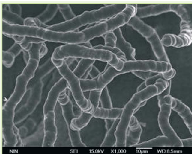
Fig. 1. Scanning Electron Microscopy image of carbon catalytic deposits
